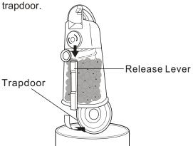
Turn the duster handle several times in the direction shown to empty the dust compartment.
